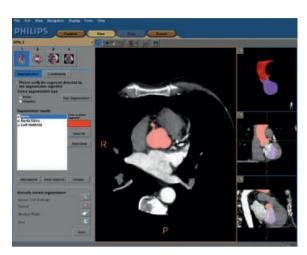
**Step 3. Import and match images.** The software automatically imports the live X-ray images. The user manually matches the 2D images with the 3D dataset.
