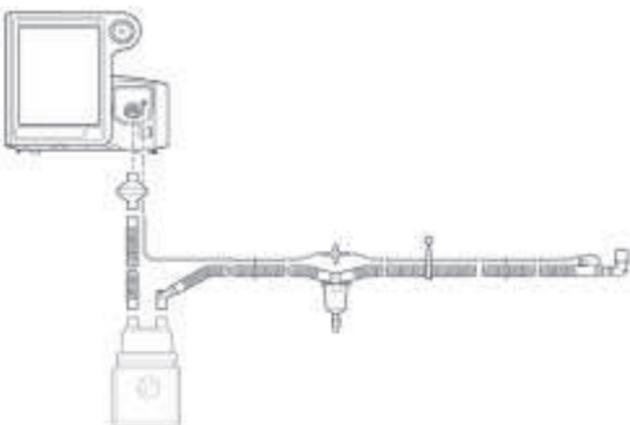
The standard humidifier patient circuit includes a main flow bacterial filter, a short tube, water trap, proximal pressure line, and elbow.
