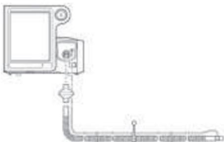
Standard patient circuit includes main flow bacterial filter and proximal pressure line. Not for use with a humidifier.
